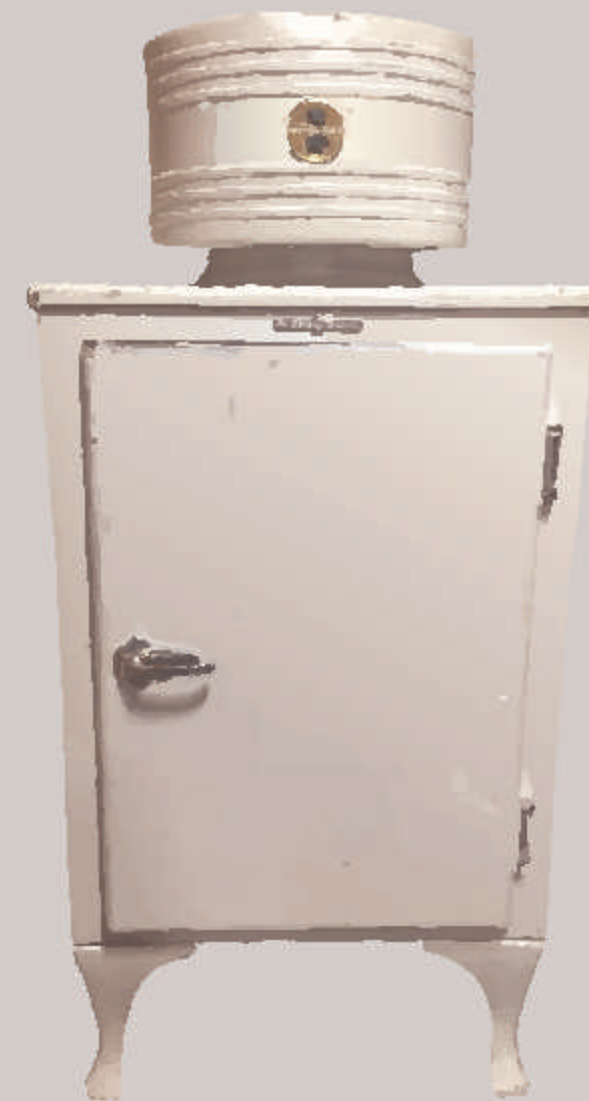
The 1930s General Electric refrigerator had a distinctive feature on top, known as the "Monitor Top". It was a condenser unit housing the compressor and condenser coils. Since the design resembled the gun turret of the Civil War ironclad ship USS Monitor, it became known as the "Monitor Top", a hallmark of General Electric's early refrigerators.
